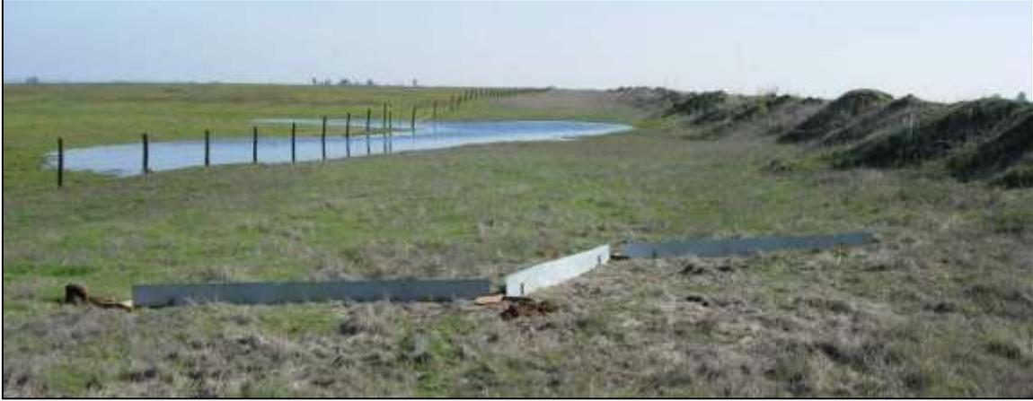
**Figure 2. Pitfall array with flashing in “Z” formation, buckets and stakes.**
