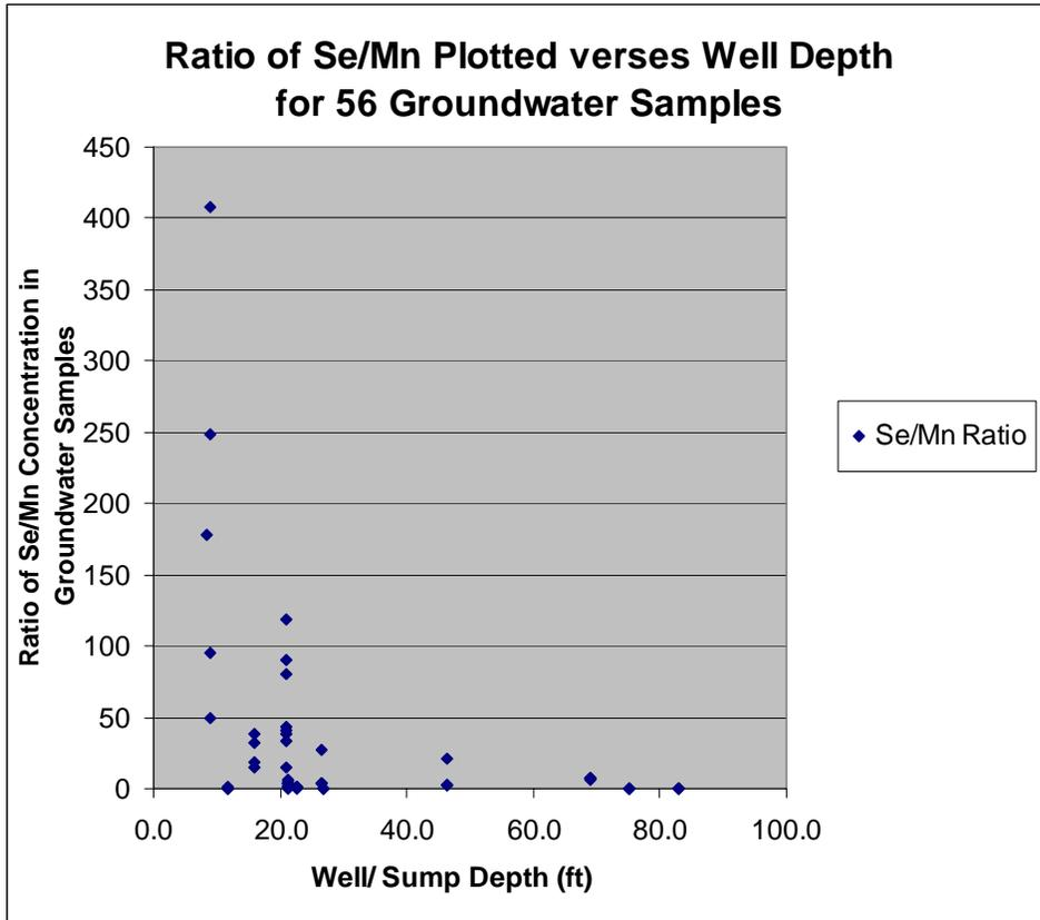
Figure 25. Ratio of Selenium to Manganese (Se/Mn) concentration in groundwater samples plotted verses well depth. The Se/Mn ratio shows a decreasing trend with depth indicating oxidizing geochemical conditions in the shallow wells and reducing conditions in the deep wells.
