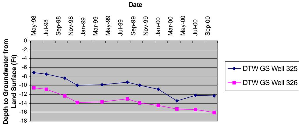
Figure 20. Hydrograph for monitor wells 325 and 326 at the Westlands Site showing typical vertical hydraulic gradient and the declining shallow groundwater trend observed.
