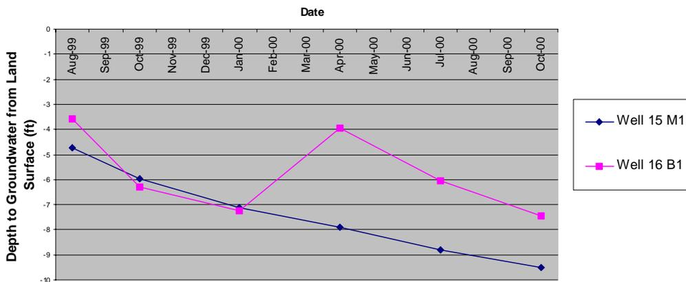
Figure 21. Hydrograph for monitor wells 15M1 and 16B1 at the Westlands Site showing an overall declining shallow groundwater trend.
