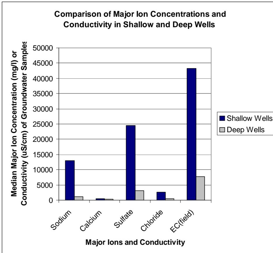
Figure 24. Comparison of dominant major ion concentrations and electrical conductivity for groundwater samples from shallow and deep wells.
