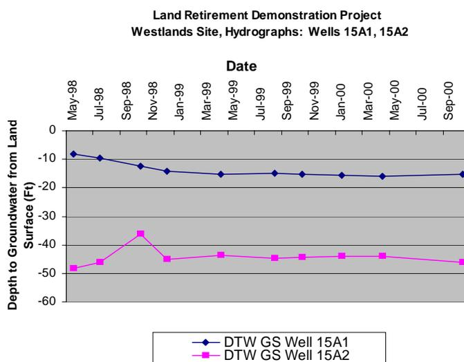
Figure 17. Hydrographs for monitor wells 15A1 and 15A2 showing typical vertical hydraulic gradients measured at the site. DTW GS = Depth to Water from Ground Surface.
