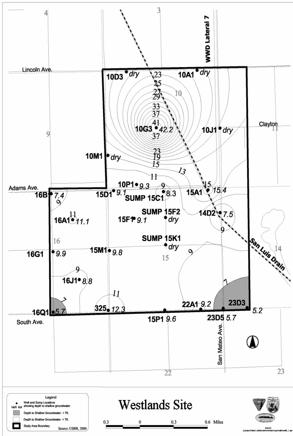
Figure 23. Depth to shallow groundwater, October, 2000. The project area underlain by shallow groundwater within 7 feet of the land surface has been reduced to approximately 55 acres.
