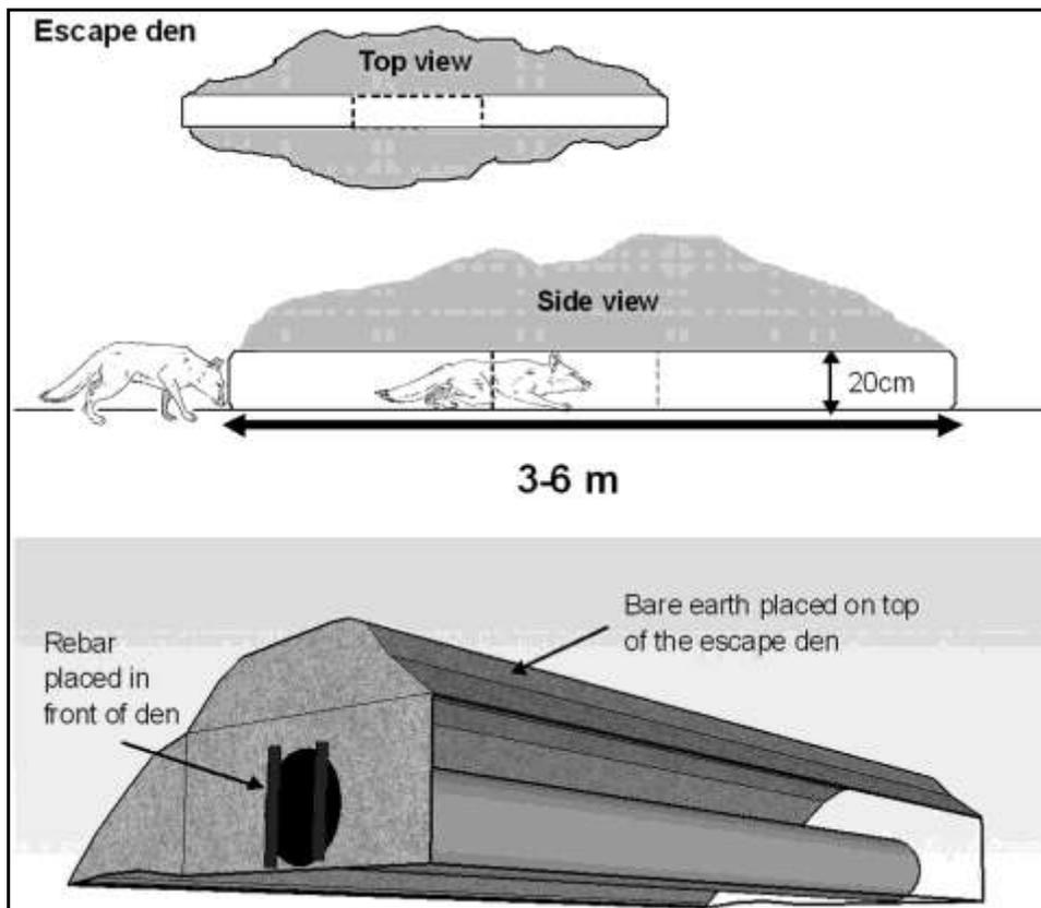
Figure 3. Schematic and field example of surface escape den for kit foxes.
