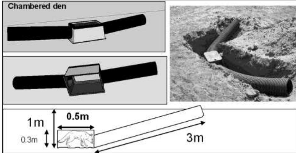
Figure 2. Schematic and field example of subterranean chambered den for kit foxes.
