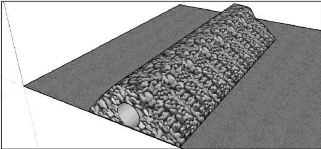
**Figure 19. Heavy substrate such as rocks can be used to cover escape dens and thus prevent livestock from exposing the structure to the elements.**
