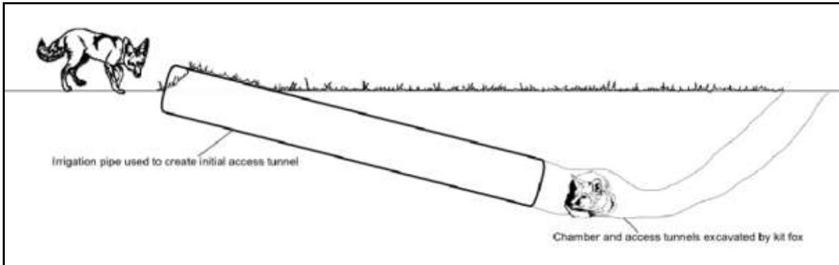
**Figure 17. Alternative den design using a single length of irrigation pipe.**
