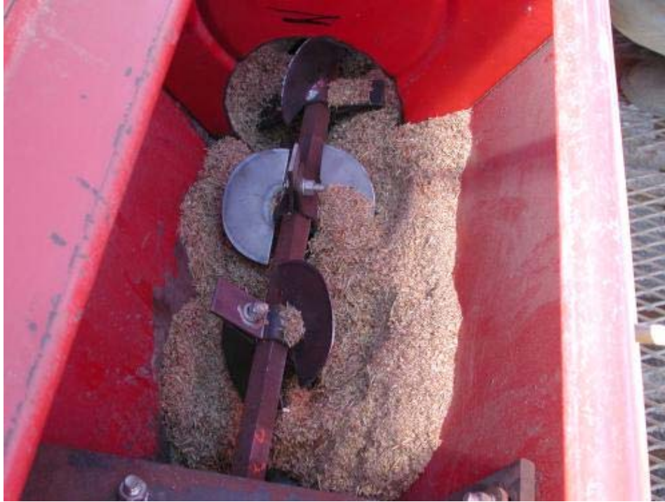
Figure 4-53. The imprinter hopper after modifications.
